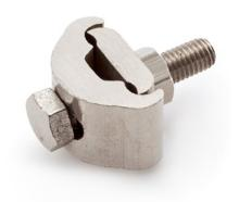
Parallel groove connector is used for connecting or branching overhead conductors. Extruded create a high strength clamp. Slotted holes allow adjusting for varying conductors on each side. its type test is accordance with IEC61238-1. Shape Body made from extruded copper or brass and bolt and spring wwasher are made of steel with hot dip galvanized plating.
